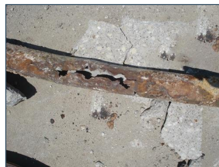
Example of corroded piping
