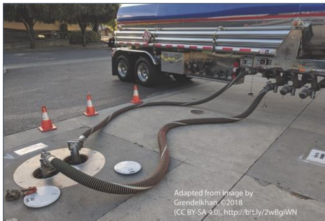
Product delivery using Stage I vapor recovery
